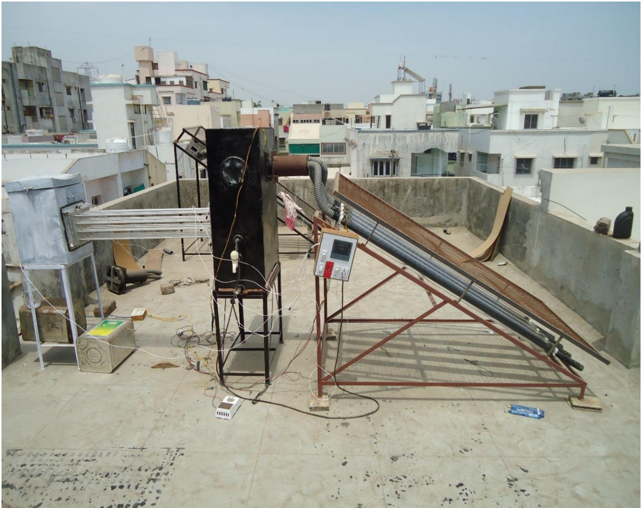
Figure 3 Practical model of humidifier & dehumidifier for (CWOA) using circular solar collector of humidification-dehumidification process
