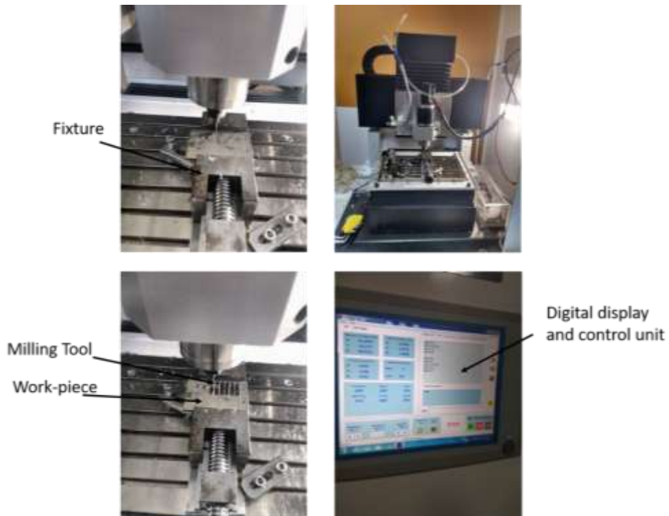
Fig. 2. Fixture assembly, milling tool, work-piece and NC control unit
