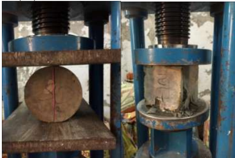
Figure 4 Compressive Strength test Machine with Specimen
