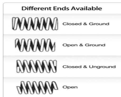
Figure 1: Types of Springs & Ends
