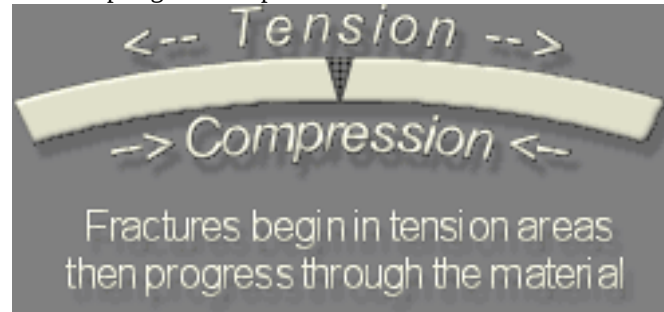
Figure 2: Tension leads to failure in bend rods
