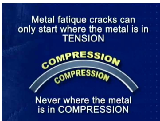
Figure 3: Inducing residual compression stress on both sides
