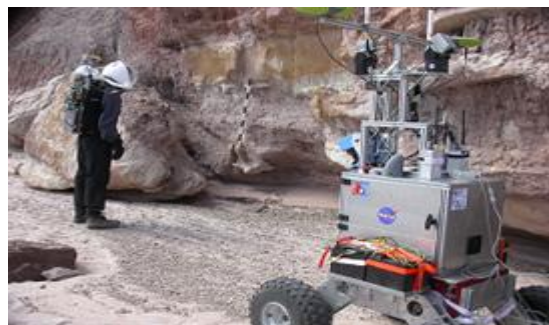
Fig 6.3 Scientist testing the software that allows wireless communication. Humans do not have to dedicate continuous attention to the robot. (Source: NASA)
