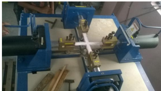
Fig 1.0 Specimen-1 held in the Bi-axial Testing Machine
