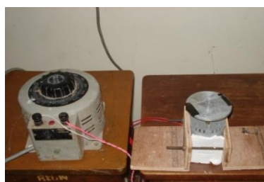
Fig 4 Fabricated Spin Coater working with motor running at max 19000 rpm
