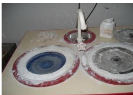
Fig 3 Conventional polishing machine for spin coating the films at low rpm
