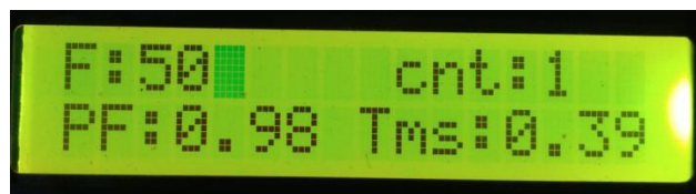
Fig. 4 LCD without power factor correction and time delay as 0.39 ms
