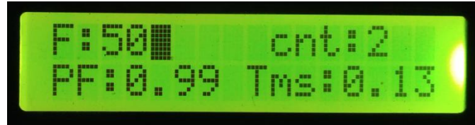
Fig. 5 LCD with power factor correction and time delay as 0.13 ms
