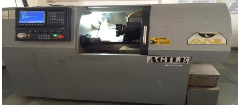
Figure 3.1CNC turning center (Photo Courtesy: S.P.B. Patel Engg College)
