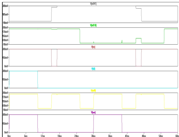
“Figure 11. Read/Write operation of 16bit 6T SRAM cell ”
