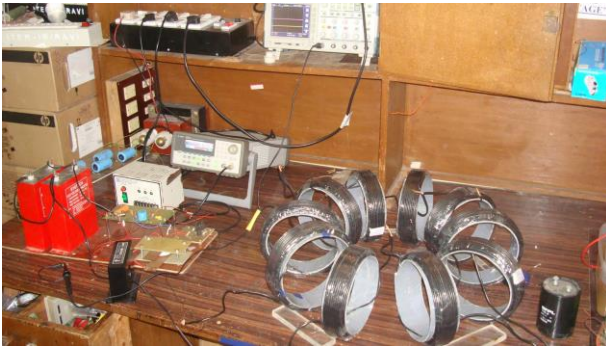
Fig. 10: Experimental setup for toroidal field coil testing.
