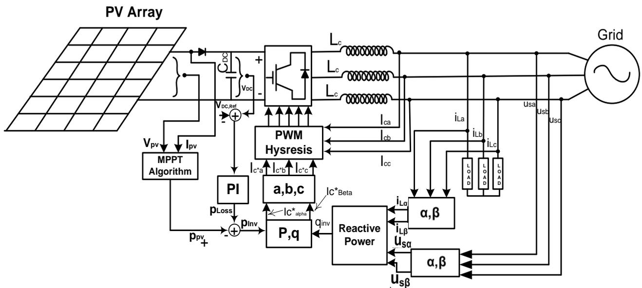
Figure 4. Block Diagram of Control Strategy of Grid Connected PV System
