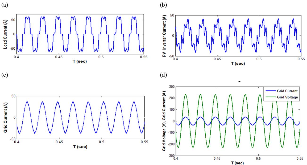
Figure 11. (a) Load Current (b) PV Inverter Current (c) Grid Current (d) Grid Voltage and Current
