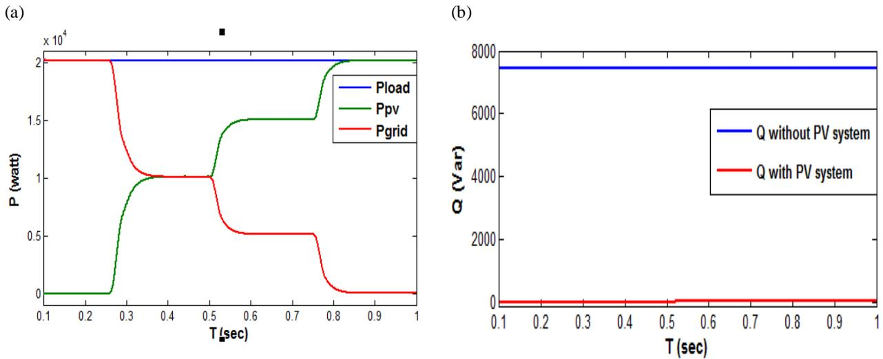
Figure 9. (a) Active Power of load, PV system and grid (b) Reactive power with and without PV system
