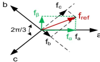
Figure 5. Transformation from a-b-c into  $\alpha$ - $\beta$  coordinates system
