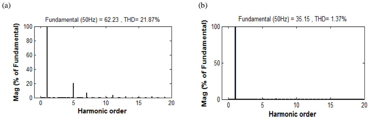
**Figure 12. Harmonic analysis (a) with and (b) without PV system**
