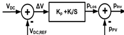
Figure 6. Block Diagram of Inverter's Active Power Control
