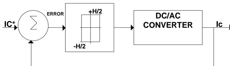
Figure 7. Block diagram of hysteresis band current control technique
