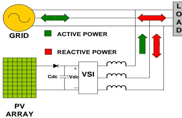
Figure 1. Proposed Grid Connected PV System
