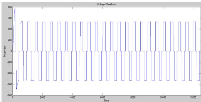
Figure2. Waveform of phase-to-phase load voltage ( $V_{ab-load}$ )
