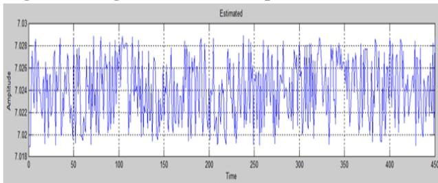
Figure42. Magnitude of 17<sup>th</sup> component of load Current
