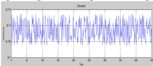
Figure18. Magnitude of 13<sup>th</sup> component of load Voltage
