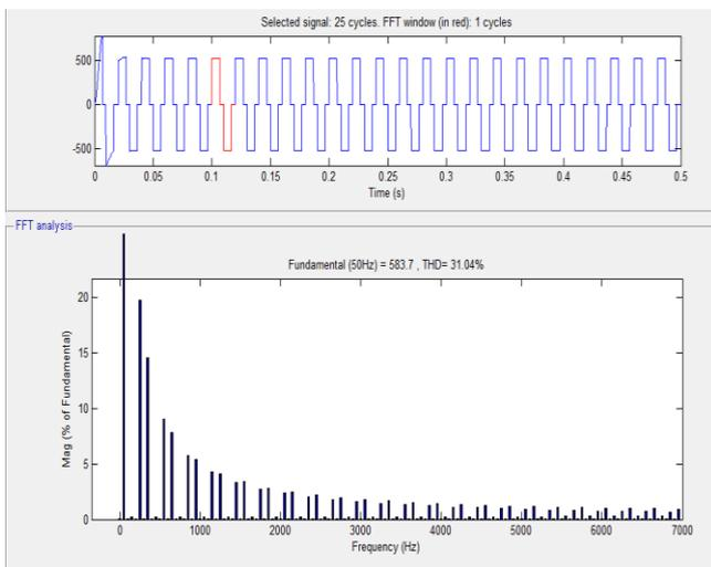
Figure4. FFT analysis of phase-to-phase load voltage ( $V_{ab-load}$ )
