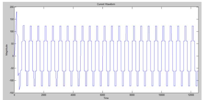
Figure3. Waveform of load current of phase a ( $I_{a-load}$ )
