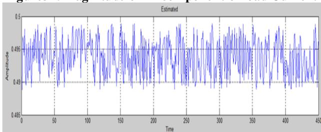
Figure34. Magnitude of 9<sup>th</sup> component of load Current
