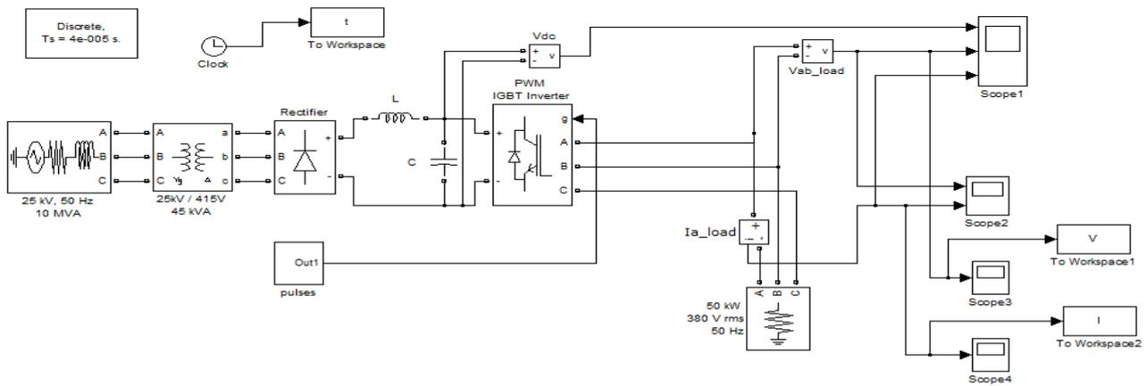
Figure1. Simulation of three phase PWM Converter
