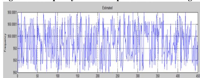
Figure25. Frequency of 19<sup>th</sup> component of load Voltage
