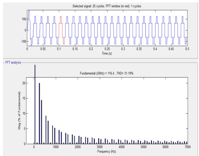
Figure5. FFT analysis of load current of phase a ( $I_{a-load}$ )
