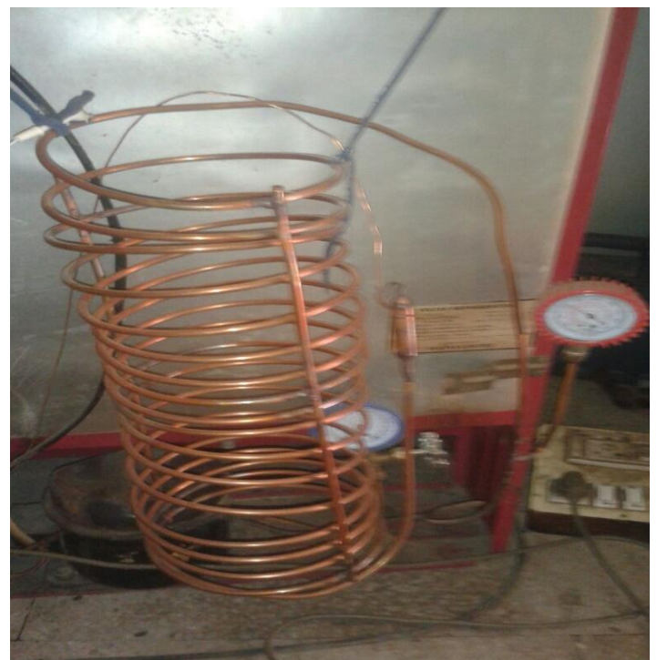
Fig. 4 Experimental Setup VCR System with helical air cooled condenser
