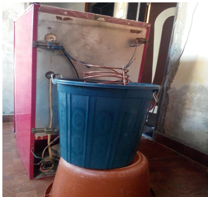
Fig. 6 Experimental setup VCR System with helical water cooled condenser
