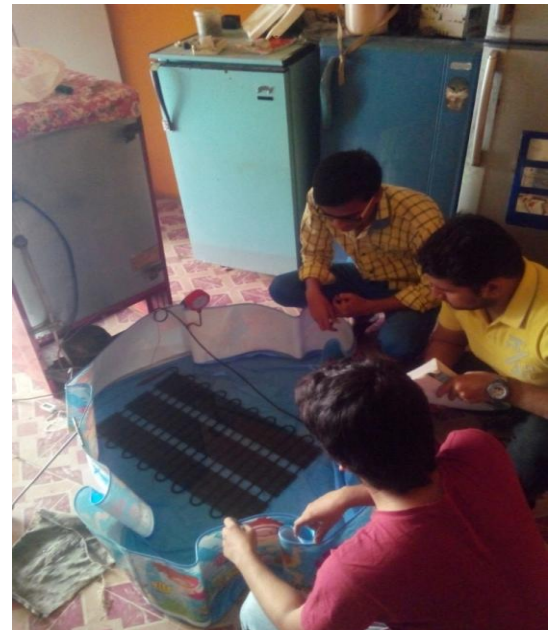
Fig. 2 Experimental Setup VCR System with water cooled condenser
