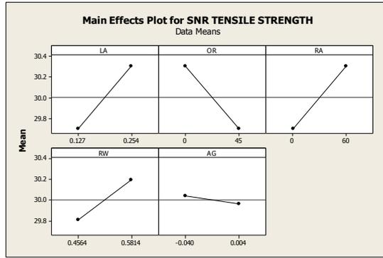
Figure 2. Effect of control factor on tensile strength
