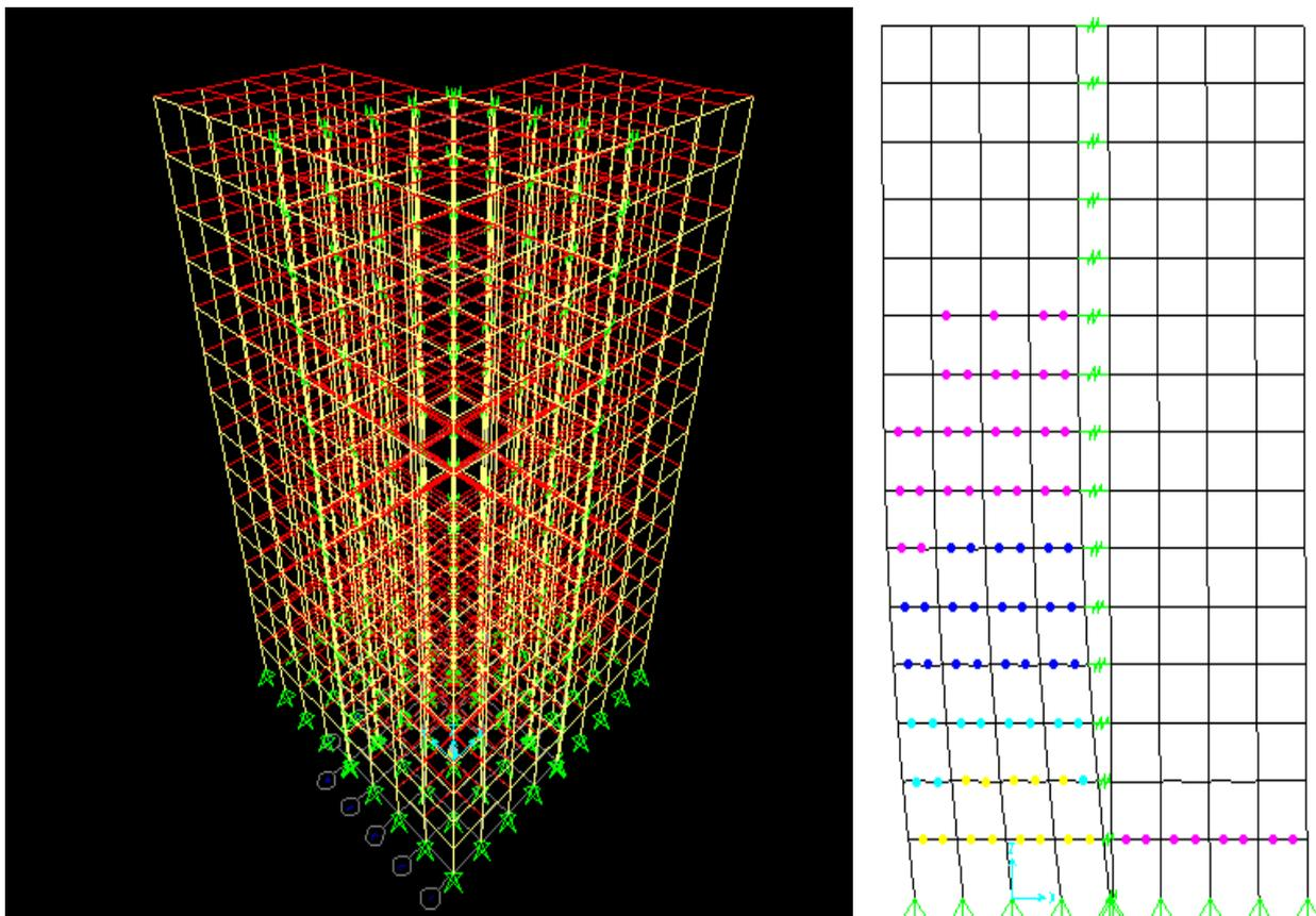
*Figure 5.1 Model and failure pattern by pushover analysis using SAP2000.*
