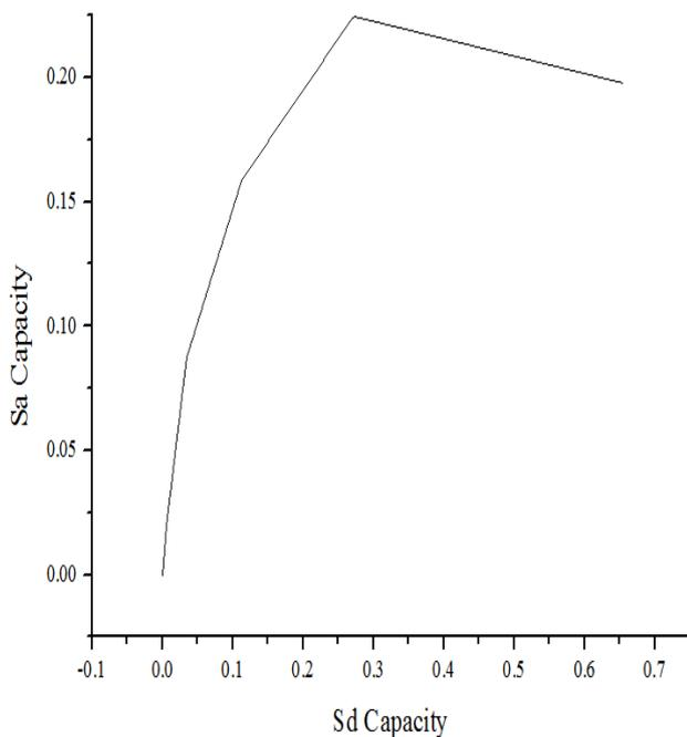
Figure 5.2 Capacity curve for 15 storey building
