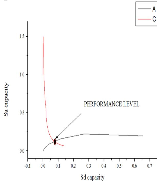
Figure 5.3 Performance level of 15 storey frame.
