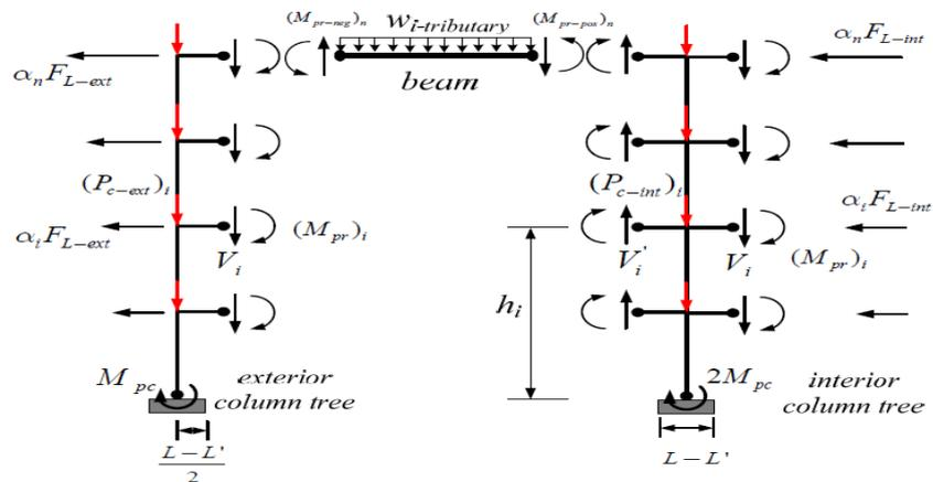
**Figure: 3.1 The free-body diagrams of beam, exterior column tree and interior column.**
