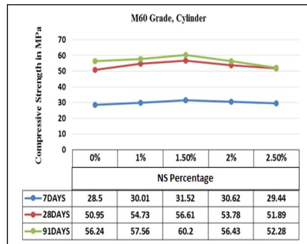
Figure 4: Compressive Strength of Cylinder M60 Grade
