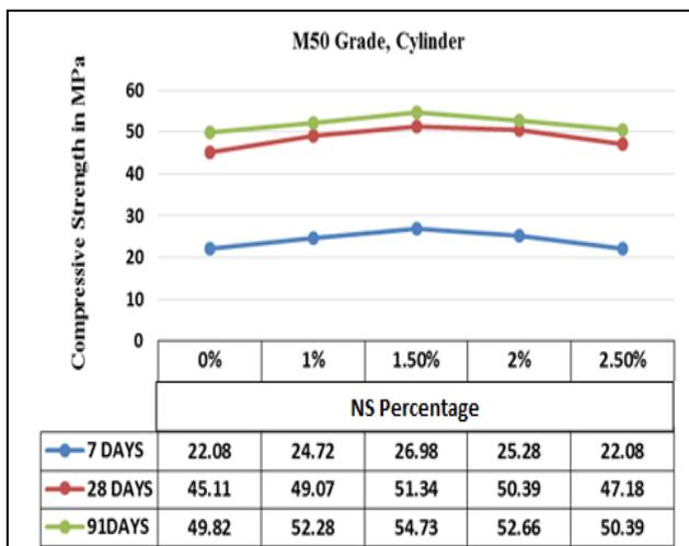
Figure 3: Compressive Strength of Cylinder M50 Grade
