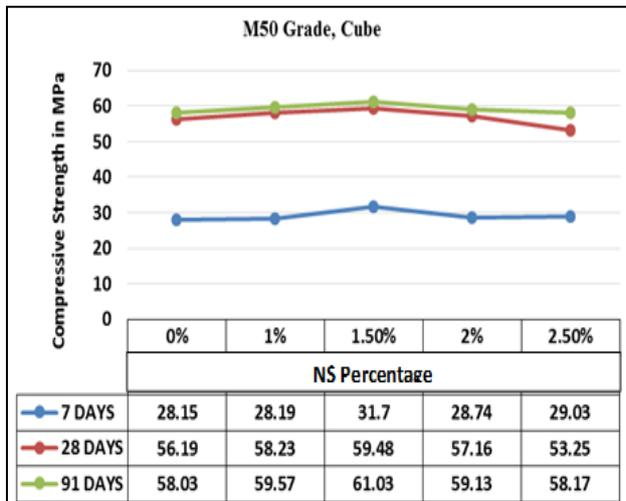
Figure 1: Compressive Strength of cube M50 Grade
