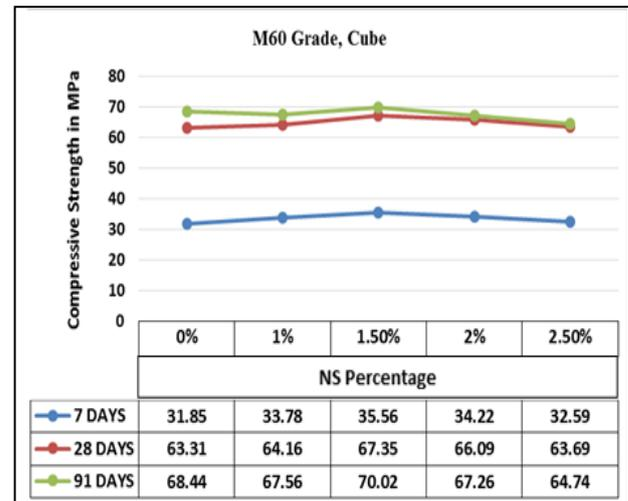
Figure 2: Compressive Strength of cube M60 Grade
