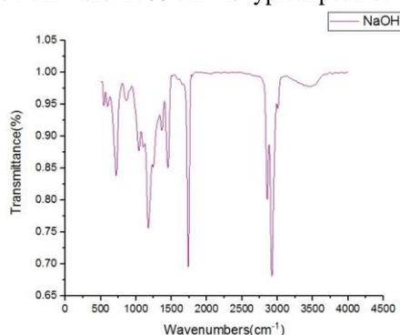
**Figure 1.4 FT-IR of NaOH**
