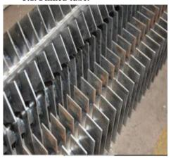
Finned tubes are used in applications involving the transfer of heat from a hot fluid to a colder fluid through a tube wall. The rate at which such heat transfer can occur depends on three factors: the temperature difference
