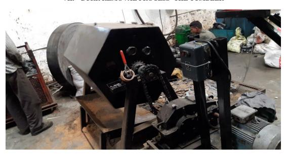
The tumbler is simply used for rotating the job with the mixture of abrasives and wood straws. It has a capacity to tumbled 1500 to 2000 jobs per turn. When the fins are made the oil which is used as a coolant remains on the fins after blanking process, so the wood straw is used for sucking the oil and to make the fins oil-free.
