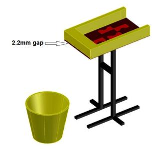
inspect the fins one needs to push the fins towards the gap. It require time and some physical work also. To eliminate this we have made improvements in this Gauge.
