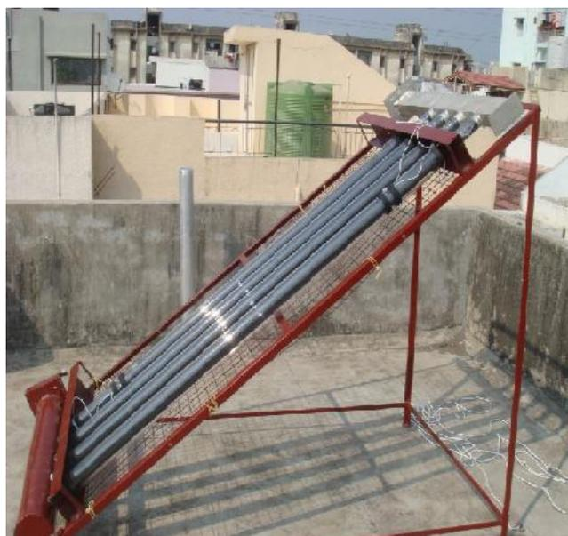
**Figure 4** Setup of circular solar air heater
