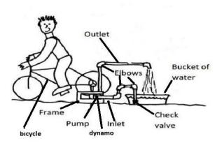
This fabricated unit consists of mainly three parts, the first one is centrifugal pump, and the third one is the stand, the third one is dynamo. This consists of a centrifugal pump operated by pedal power. The centrifugal pump is positioned on its stand in such a way that driven shaft of the centrifugal pump is butted to the bicycle wheel. By pedalling the bicycle,
