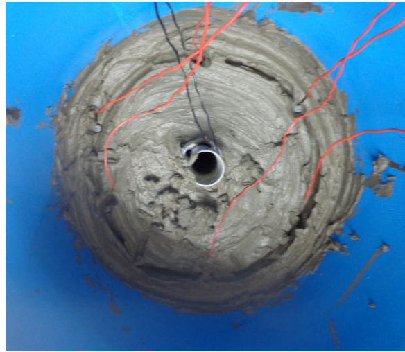
Fig. 8 Nonwoven Conductive drain (Cathode)
