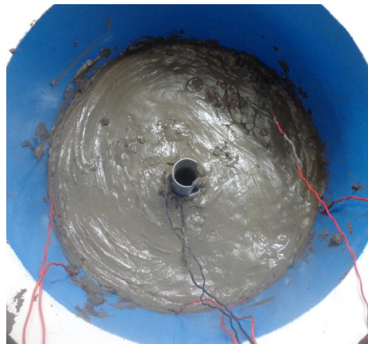
Fig. 6 Conductive drain with PVC pipe
