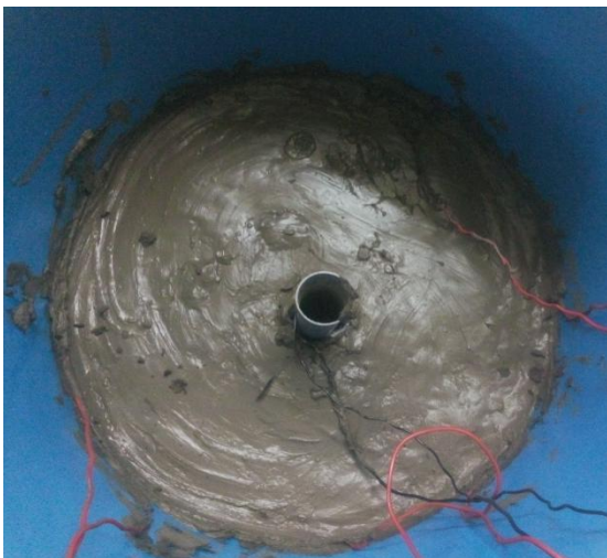
Fig. 5 Insertion of PVC pipe
