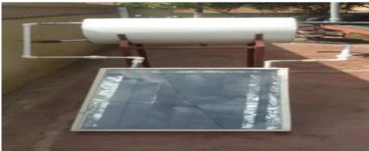
**Eze J. I. and Ojike O. (2012) [2]** investigated the thermal efficiency of a passive solar water heater is undertaken. The solar water heater has two storage tanks and is used for cold and warm waters, respectively. Here copper pipes are placed in the spiral form only.
