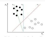
$\rm H_1$  does not separate the classes.  $\rm H_2$  does, but only with a small margin.  $\rm H_3$  separates them with the maximum margin.
