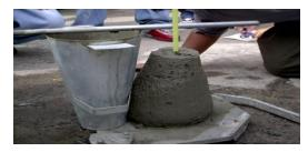
Fig-6: Slump of fresh concrete measured.
