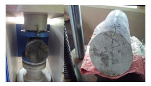
Fig-8: Tensile strength of concrete cylinder and failure pattern
