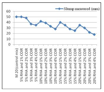
Chart-1: Slump test result of fresh concrete.
