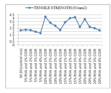
Chart-3: Tensile strength test result
