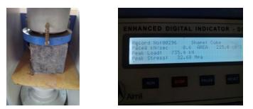
Fig-7: Compressive strength on cube and its result.
