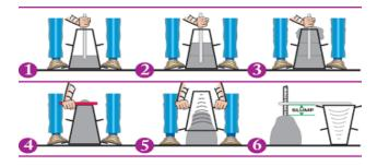
Fig-5: Procedure of measuring slump of fresh concrete.
