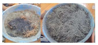
Fig-4: Cement mixed with Rice-husk ash and COIR fiber
