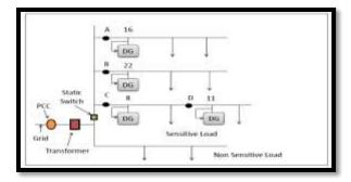
Fig.1 Basic Micro-grid Architecture
