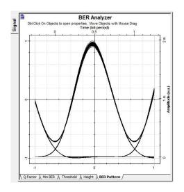
Figure 1: Eye Diagram for 8 Channels & 5dbm Input Power
