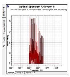
Figure 6: Input Spectrum for 16 Channels & 10 dbm Input Power
