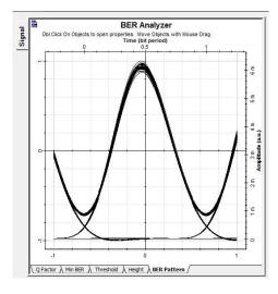
Figure 2: Eye Diagram for 16 Channels & 10dbm Input Power
