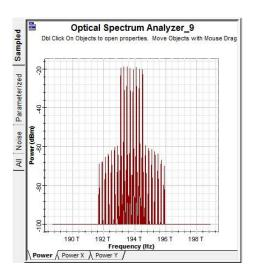
Figure 5: Output Spectrum for 8 Channels & 5 dbm Input Power
