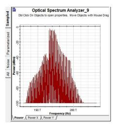
Figure 9: Output Spectrum for 32 Channels & 20 dbm Input Power
