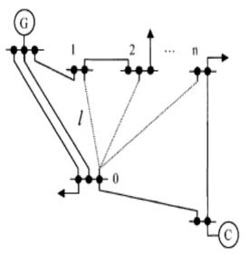
Fig. 1 Concept of branch topology identification.
