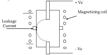
In this system, the open contacts of VI bottle are subjected to high Voltage DC supply to establish the capacitance between two contacts.
