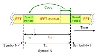
Fig. 4 Addition of a guard period to an OFDM signal.
