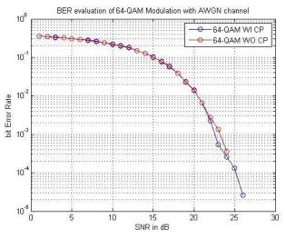
Fig. 8 Comparison of 64-QAM with & without cp
