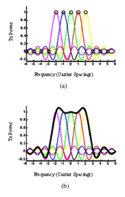
Fig. 2 Frequency response of the sub carriers in a 5 tone OFDM signal
