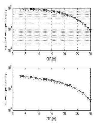
Fig 5:- Output of STBC with awgn channel
