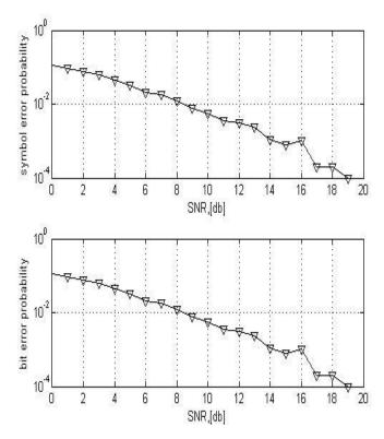
Fig. 6 Output of 2\*2 MIMO-OFDM using STBC with Rayleigh channel
