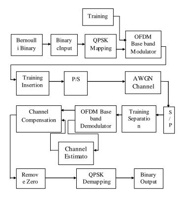
Fig. 3 Block diagram showing a basic OFDM Transceiver.
