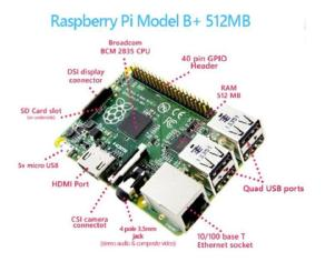
Figure 2: Raspberry Pi B+ Board
