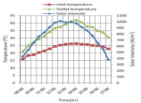
Variation of outlet temperature inlet temperature and solar intensity with time for stainless steel sheer reflector.
