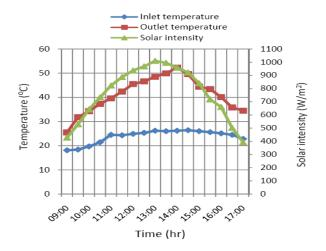
Variation of outlet temperature, inlet temperature and solar intensity with time for stainless Aluminum foil as reflector
