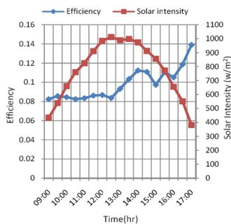
A.Variation of Solar Intensity and Temperature with Time for Aluminum Sheet as Reflector:-
