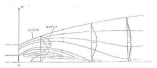
"Fig. 7" Typical profiles of axial and swirl velocity components in a strongly swirling flow
