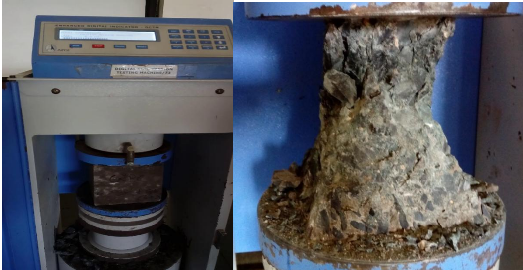
Figure 1: Compressive strength test
