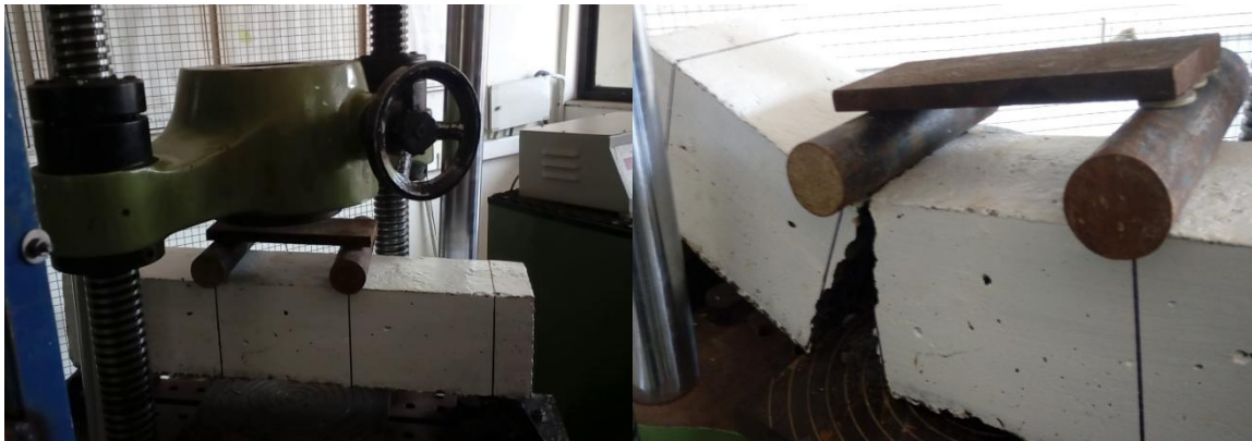
Figure 5: Flexural strength test
