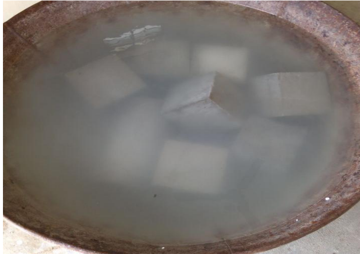
Figure 5. Curing of the moulded concrete blocks
