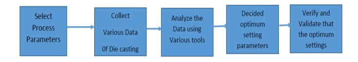
Figure-1 Steps of Taguchi method in Die Casting Process
