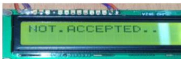
FIG: DISPLAYING THAT UNAUTHORISED PERSON TRY TO OPEN THE DOOR
