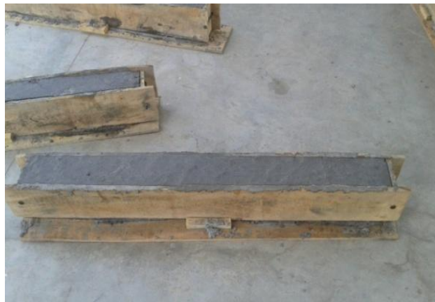
Fig 4 Formwork with Beam Specimen
