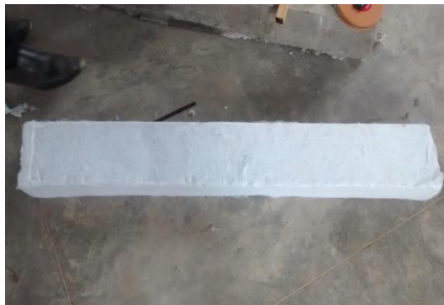
Fig 5 External Wrapping by white cement
