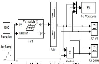
Figure 2. Matlab model of single PV array
