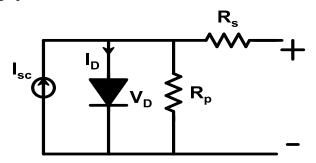
Figure 1. PV Cell internal circuit
