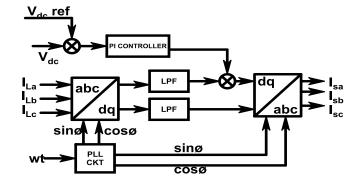
Figure 4. . Block diagram of SRF control algorithm
