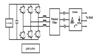
Fig.5. PV system connected to grid with 3-ph inverter
