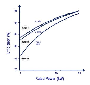
Fig 1.2 – Curves Efficiency – Rated Power
