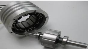
In order to operate with low speeds, a high number of Fig 3.1 Model of PMSG poles is used in PMSG wind turbines. Instead of electrical DC excitation the magnetic rotor field is IV. MPPT CONTROL ALGORITHM
