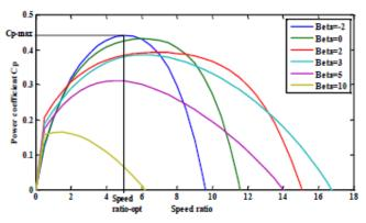
Fig 2.2Power coefficient values at different speeds
