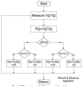
Fig 4.2Perturb and Observe Algorithm
