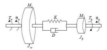
Fig 2.3 Two Mass Drive Train Model
