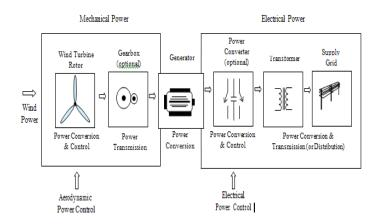
Fig 2.1 AgenericWindEnergyConversionSystem
