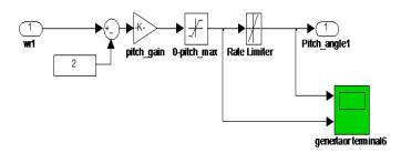
Fig 2.5Simulink Model of Pitch Angle Controller
