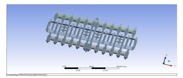
Fig. 1.4, 3 D Model of Plastic Slat Belt
