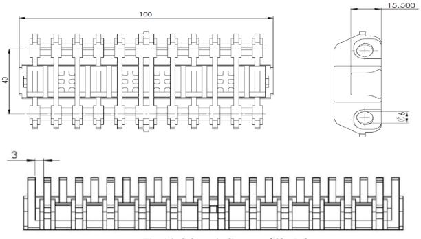
Fig. 1.3, Schematic diagram of Slat Belt
