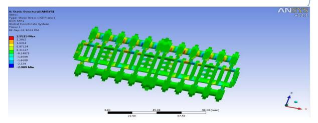
Fig. 1.9, Shear Stress
