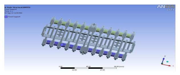
Fig. 1.6, Applying fixed support
