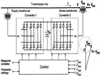
Fig. 1 : Basic circuit arrangement of UPFC
