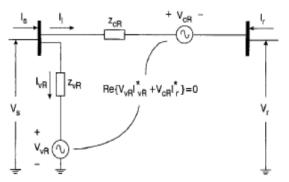
Fig. 2 : Equivalent source of UPFC voltage source-based model
