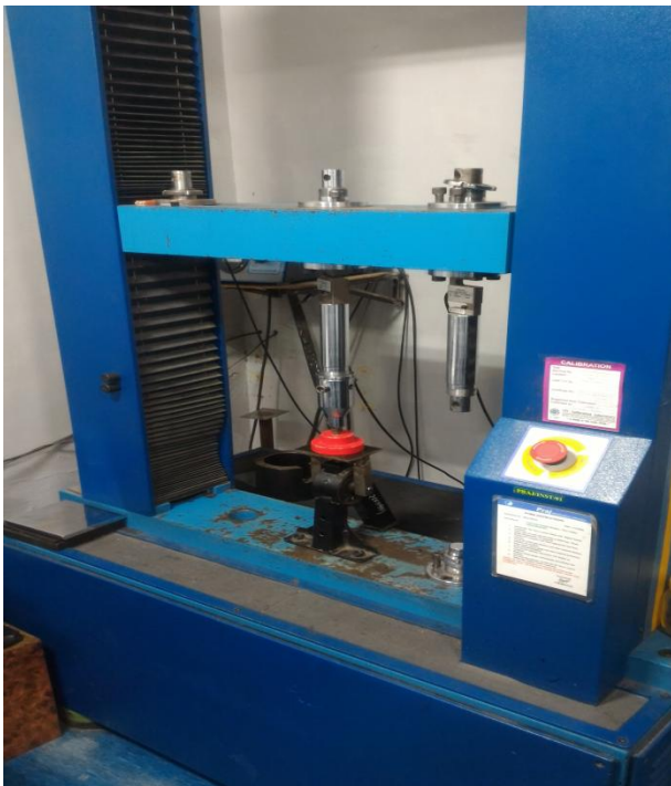
Fig. 6. UTM in loading condition
