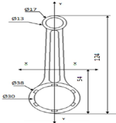
Fig.2: Dimensions for Bajaj Pulsar 150cc Engine connecting rod
