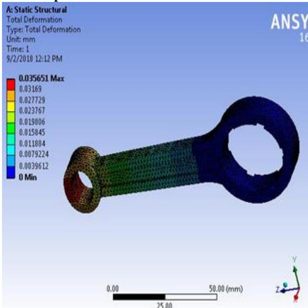
Fig.8: Total deformation of connecting rod
