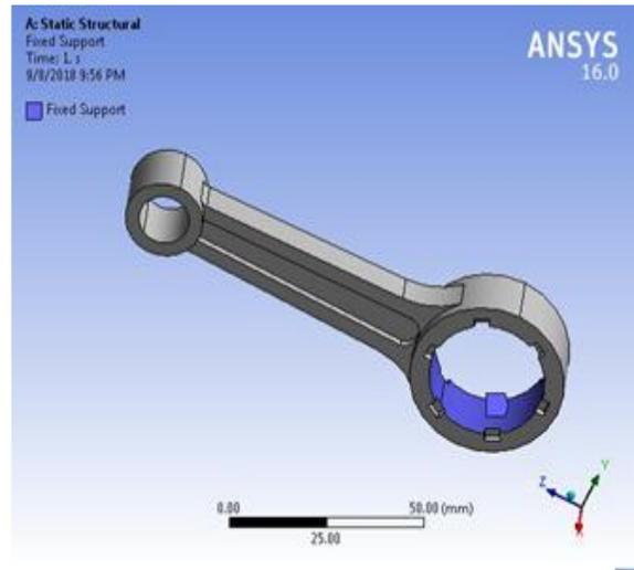
Fig.7: Constraint for connecting rod
