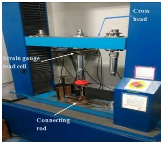
Fig.10: Experimental setup
