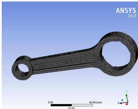
*Fig.5: Meshed model of connecting rod*
