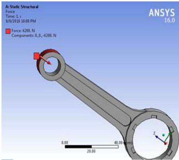
Fig.6: Force on connecting rod
