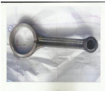
**Fig.1: Existing connecting rod**
