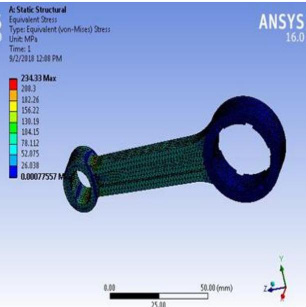
Fig.9: Equivalent stress on connecting rod
