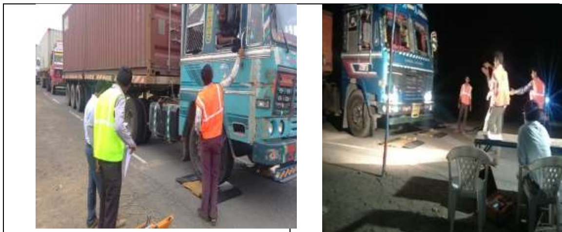
Photos_1: Axle Load Survey at Km 196/200 of SH-36
