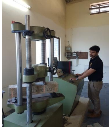
Fig 7. Three point load test on beam
