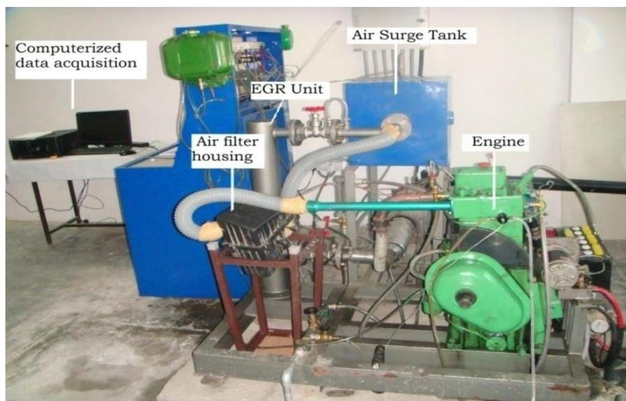
**Fig: 2.2** Photographic View of Computerized Diesel Engine Setup with Air Filter Housing Arrangements and EGR Facility
