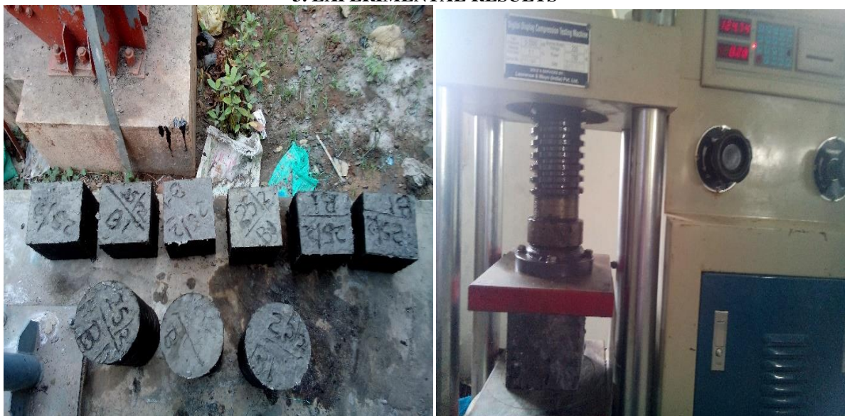
Fig 2: Casted and Testing of Basalt Concrete Cubes
