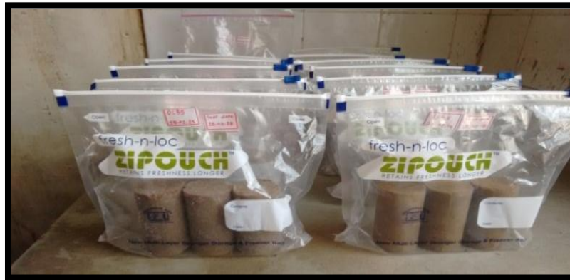
Figure 1 Moisture Retaining Technique used for UCS Samples
